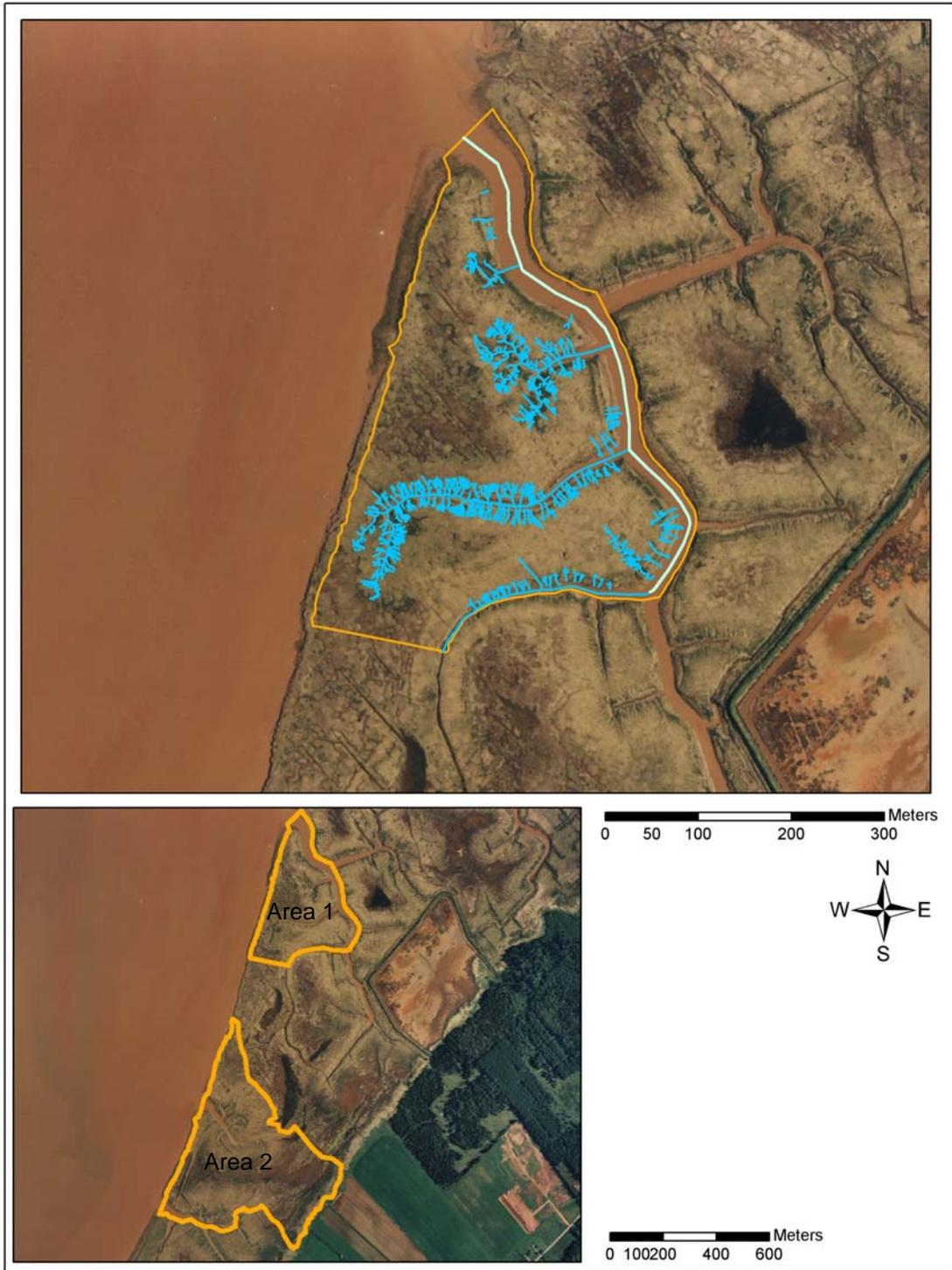
**Figure 4:** Aerial photograph (1:10,000) taken in 1995 showing field surveyed tidal channel network in blue and boundaries of study sites (orange) at study area 1 of John Lusby marsh. (Photo source: Dept. of Natural Resources, 1995)
