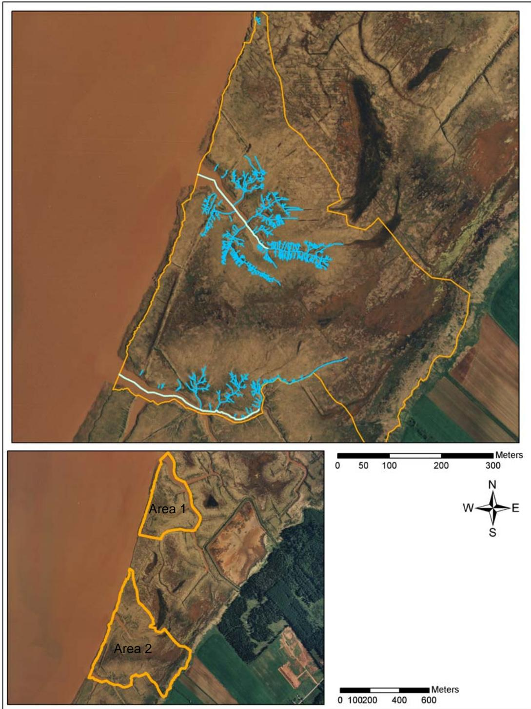
**Figure 5:** Aerial photograph (1:10,000) taken in 1995 showing field surveyed tidal channel network in blue and boundaries of study sites (orange) at study area 2 of John Lusby marsh. (Photo source: Dept. of Natural Resources, 1995)
