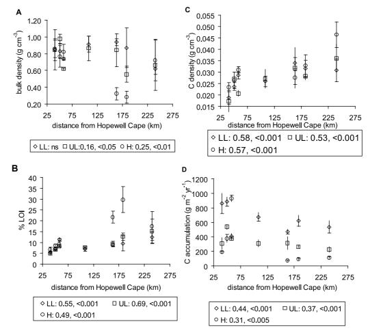
**Figure 3.** Relationship of marsh distance from Hopewell Cape to average: (a) bulk density, (b) %LOI, (c) carbon density, and (d) rate of carbon accumulation in the lower low marsh (LL), upper low marsh (UL), and high marsh (H) in tidal salt marshes along the Bay of Fundy coast. The first number in the legend is  $r^2$ ; the second is the probability. Vertical bars represent  $\pm 1$  standard deviation.
