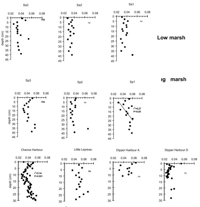
Figure 8. Carbon density (g cm<sup>-3</sup>) with depth from cores taken in tidal salt marshes in the outer Bay of Fundy.
