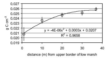
**Figure 4.** Carbon density of soils collected along a high-marsh transect at Belliveau Village, New Brunswick. Points represent average of three samples, and vertical bars represent  $\pm 1$  standard deviation.
