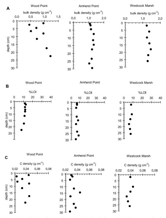
Figure 7. (a) Bulk density, (b) LOI, and (c) carbon density in soils from marshes in the upper Bay of Fundy.
